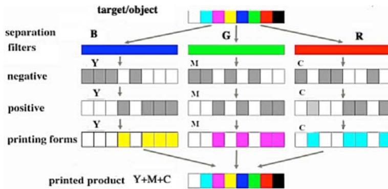
Fig. 1: principle of preparing basic C-M-Y separations
