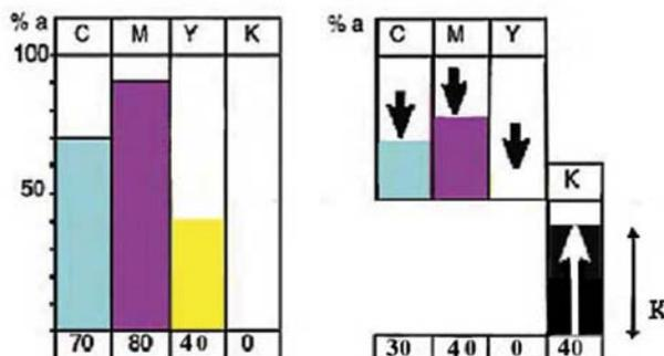
Fig. 6: example of a pair of NIR twins: pure CMY combination (left), interchanged K content (right)
