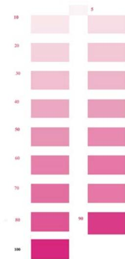
Fig. 7: series of magenta patches coverages from 10-90 % in 10 % step (left), 5% shift (right)
