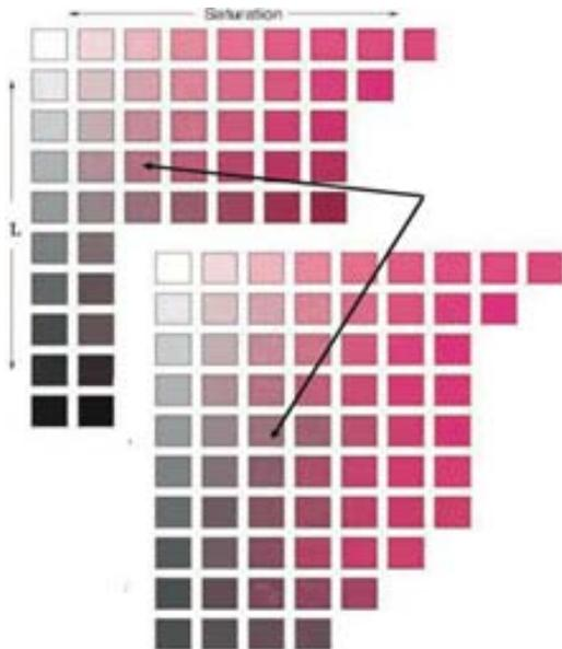
Fig.7: two hue patches arrangement varying L and S, plotted as CMY and CMY+K combinations (example)
