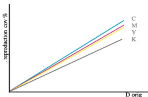
Fig.1b: four color reproduction curves (CMY+K), schematic
