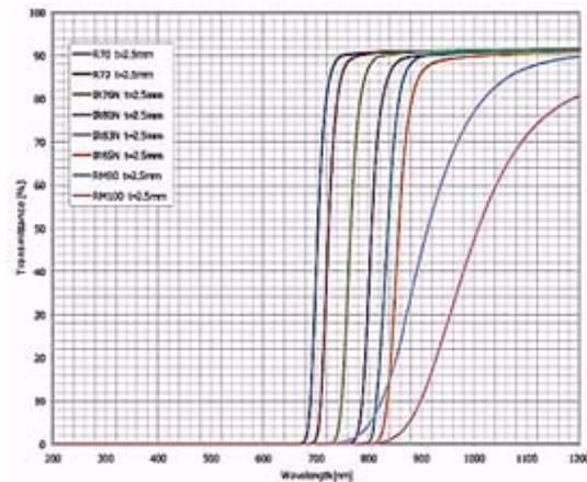
Fig. 4: NIR domain transmittance filter series
